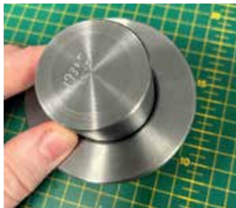
SHAFT ALIGNED READY FOR PRESSING
