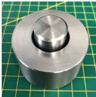
SHAFT FITTED INSIDE BORE
