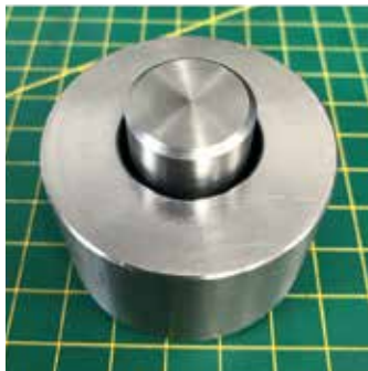
SHAFT ALIGNED READY FOR PRESSING
